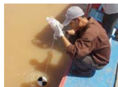
The boat used for sampling; sampling turbidity using a sechi disk; and sample analysis on board the boat
